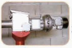
An electric motor with automatic feed level sensor will ensure continuous feed availability in the feeding lines hoppers.
